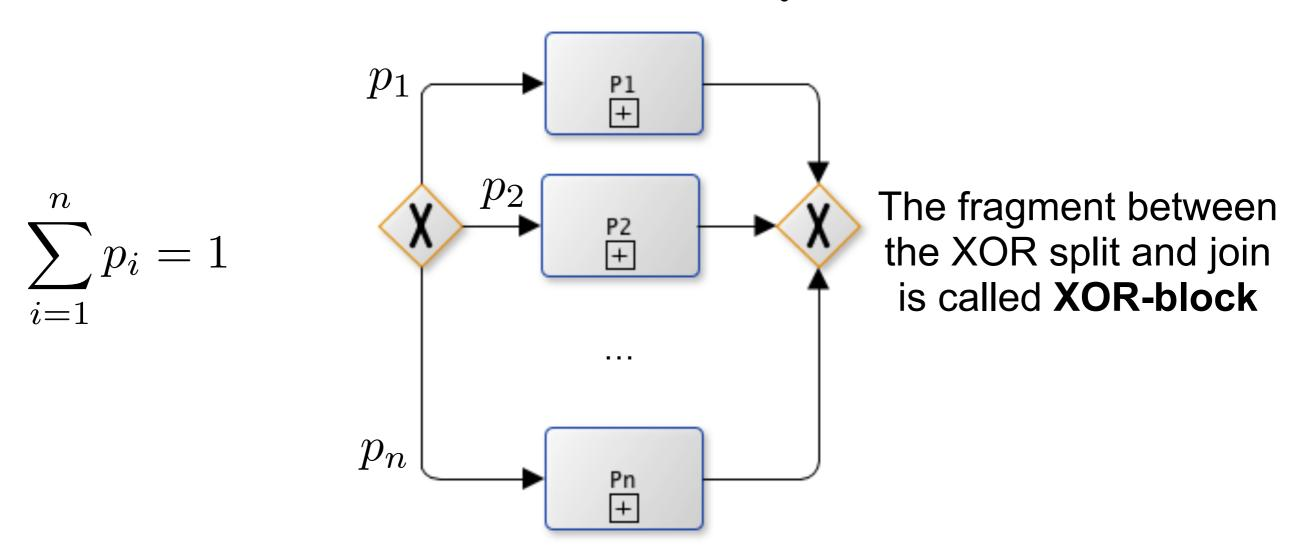
The cycle time of a XOR-block fragment is the **weighted average** of the cycle times of the branches
