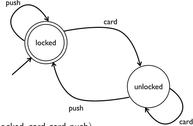
$\delta({\sf locked}, {\sf card}) = {\sf unlocked}$   $\delta({\sf locked}, {\sf push}) = {\sf locked}$   $\delta({\sf unlocked}, {\sf card}) = {\sf unlocked}$  $\delta({\sf unlocked}, {\sf push}) = {\sf locked}$   $\widehat{\delta}(\mathsf{locked},\mathsf{card}\;\mathsf{card}\;\mathsf{push})$
