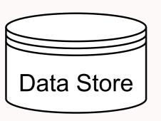
A **Data Store** is a place where the process can read or write data, e.g., a database or a filing cabinet. It persists beyond the lifetime of the process instance.
