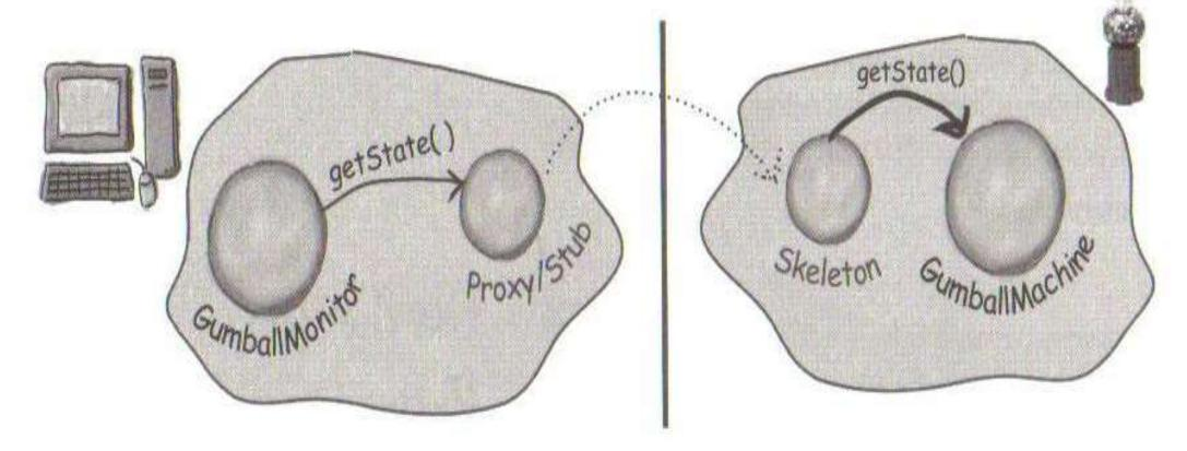
GumballMachine returns the state to the skeleton, which serializes it and transfers it back over the wire to the proxy. The proxy describilizes it and returns it as an object to the monitor.
