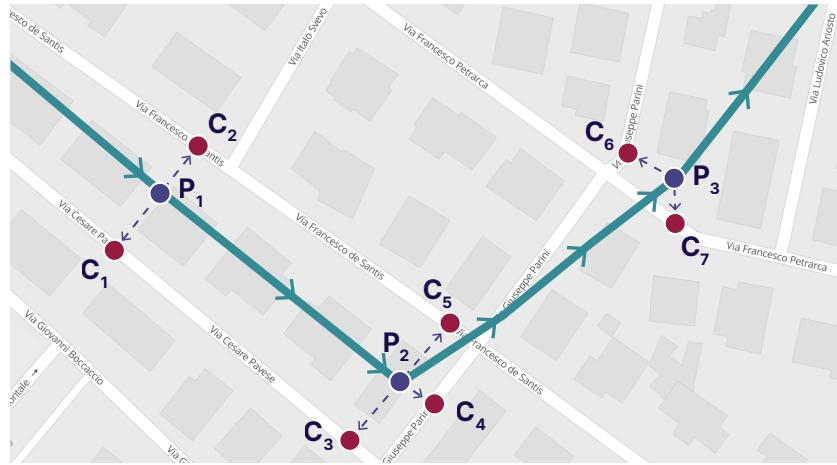
Figure 4.6 Sample raw trajectory with three points ( $P_1, P_2, P_3$ ) and the corresponding candidate projections on neighboring segments ( $C_1, \dots, C_7$ ). (Background map taken from OpenStreetMap, MapTiler OMT layer)
