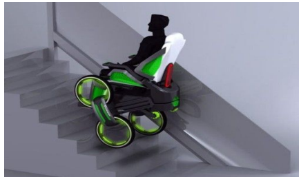
Figure: iBOT - Robotic stair climbing wheelchair [5]
