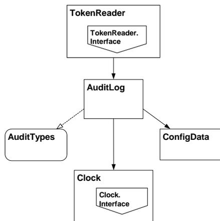
**Figure 8 : The Second SPARK Subsystem**
