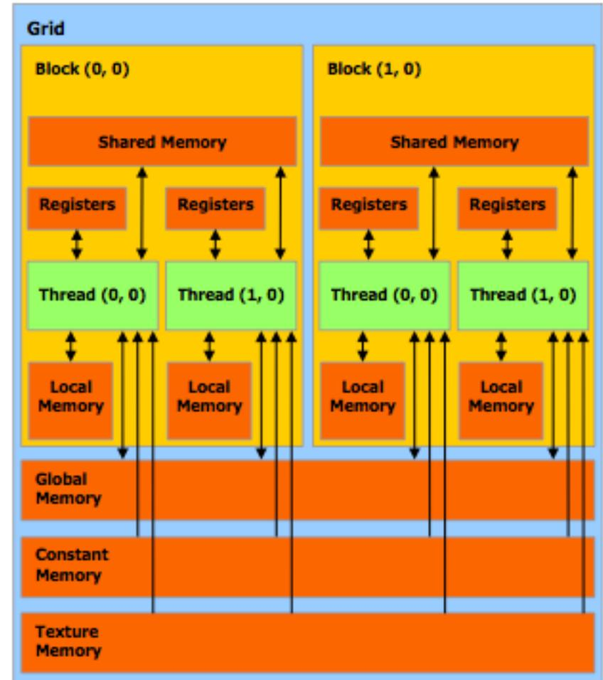
A thread has access to the device's DRAM and on-chip memory through a set of memory spaces of various scopes.
