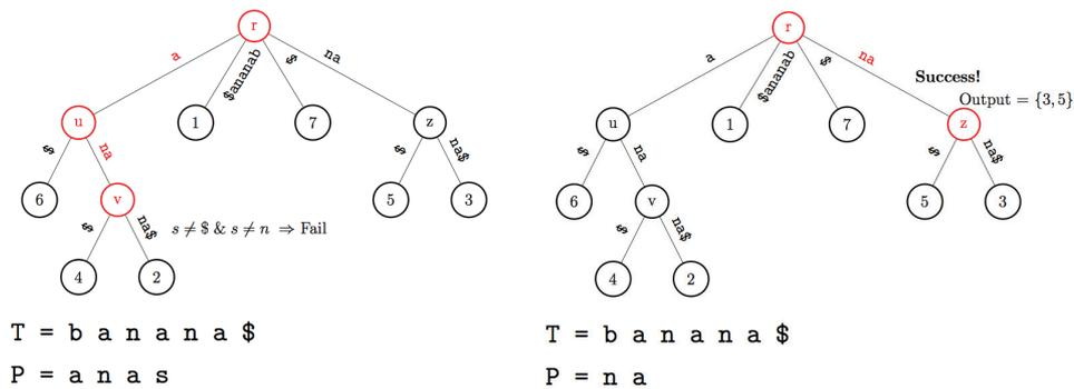
FIGURE 8.9: Two examples of substring searches over the suffix tree built for the text  $\text{banana}\$$ . The search for the pattern  $P = \text{anas}$  fails, the other for the pattern  $P = \text{na}$  is successful.
