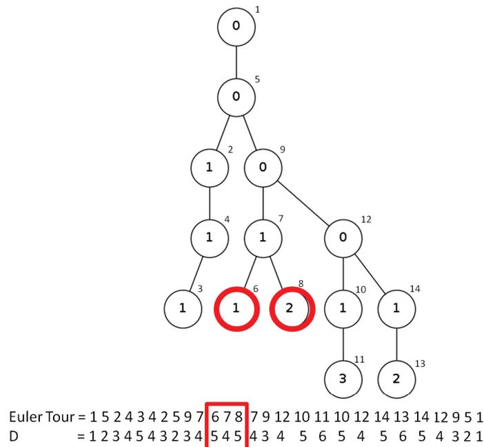
FIGURE 8.14: Cartesian tree built on the  $lcp$ -array of Figure 8.12. On the bottom part are reported the Euler Tour of the Cartesian Tree and the array  $D$  of the depths of the nodes according to the Euler-Tour order.
