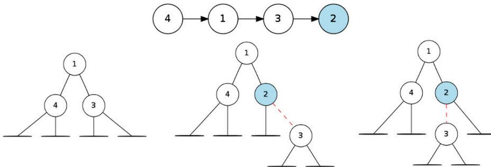
FIGURE 8.13: Example of Cartesian Tree built over the array  $A[1, 3] = \{1, 4, 3\}$ , and the insertion of the value 2. Observe that nodes of  $C_A$  store only  $A$ 's values, their positions in  $A$  are dropped to ease the presentation.
