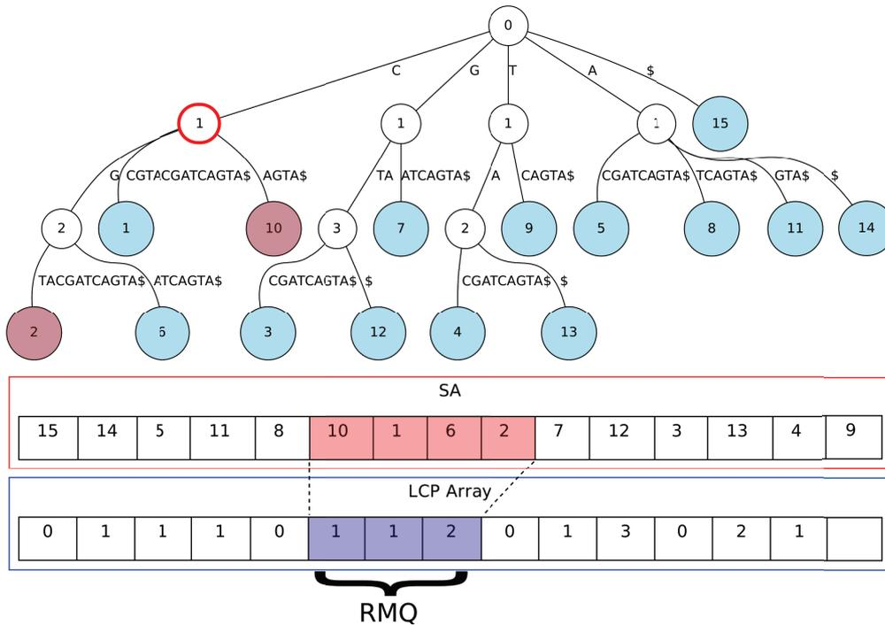
FIGURE 8.12: An example of suffix tree (unordered), suffix array, lcp-array for the string  $X = \text{CCGTACGATCAGTA}$ . The figure highlights that the computation of  $\text{lcp}(X[2, 16], X[10, 16])$  boils down to finding the depth of the lca-node in  $ST_X$  between the leaf 2 and the leaf 10, as well as to solve a range minimum query on the sub-array  $\text{lcp}[6, 8]$  since  $SA_X[6] = 10$  and  $SA_X[9] = 2$ .
