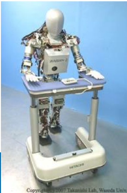
WABIAN testing the Walking Aid Robot for Elderly developed by HITACHI (WABOT-HOUSE Project, Gifu Prefecture)
