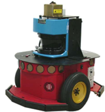
Map building using the LMS 200 laser scanner
