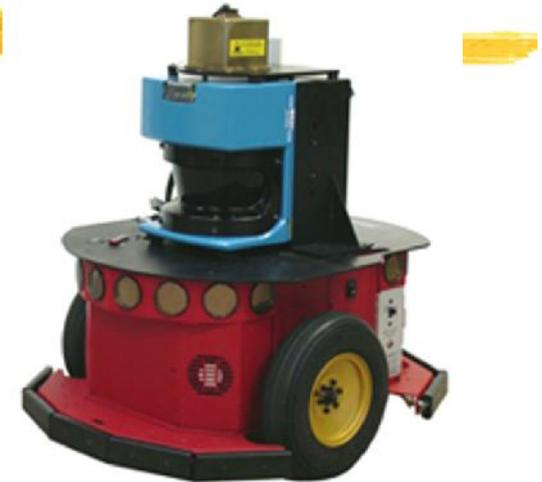
Map building using the LMS 200 laser scanner
