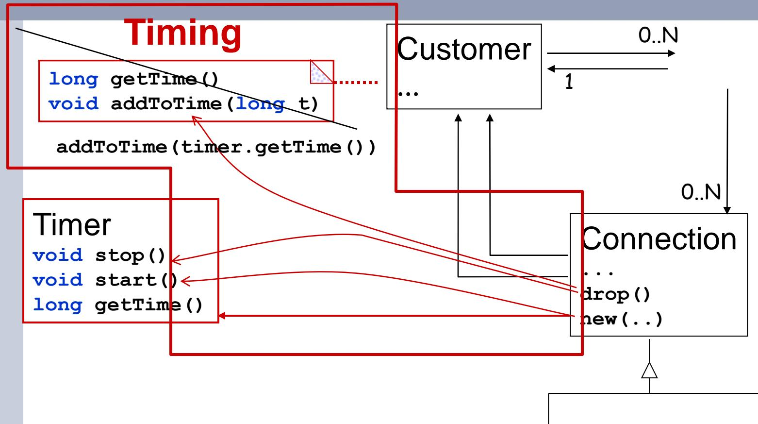
timing as an aspect captures the protocols involved in implementing the timing feature
