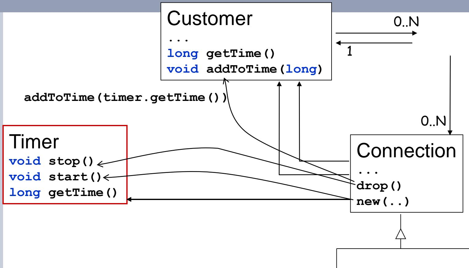
timing as an object captures timing support, but does not capture the protocols involved in implementing the timing feature
