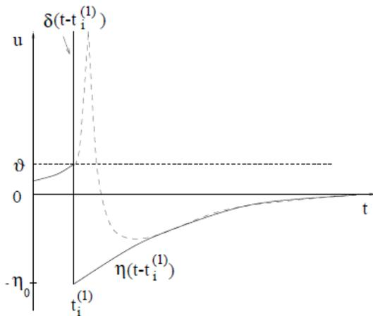
$$\eta(t - t_i^{(f)}) = \begin{cases} 1/\Delta t & \text{for } 0 < t - t_i^{(f)} < \Delta t \\ -\eta_0 \exp\left(-\frac{t-t_i^{(f)}}{\tau}\right) & \text{for } \Delta t < t - t_i^{(f)} \end{cases}$$
